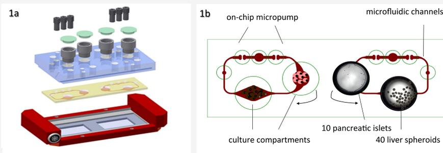
**Fig. 1. The microfluidic 2-OC device at a glance.** a) Exploded view of the device comprising a polycarbonate cover-plate (blue), the PDMS-glass chip accommodating two microfluidic circuits (yellow; footprint: 76 mm x 25 mm; height: 3 mm) and a heatable MOC-holder (red) b) Experimental Set up with 40 liver spheroids co-cultured with 10 human pancreatic islets to investigate insulin-glucose cross-talk in the 2OC.
