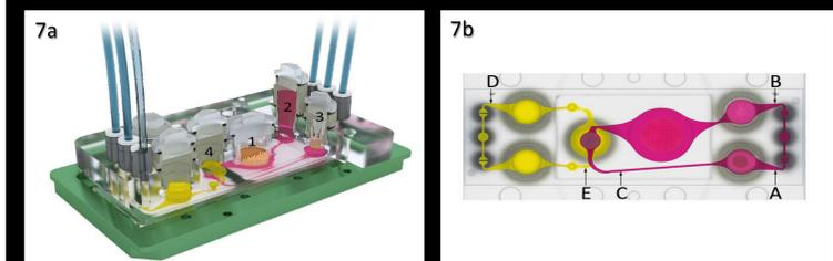
**Fig. 7. The microfluidic 4-OC device at a glance.** a) 3D view of the 4OC device with culture compartments for intestine (1), pancreatic islets (2), liver (3), and kidney (4) tissue b) Top view of the four-organ-chip layout (footprint: 76 mm x 25 mm; height: 3 mm) accommodating a surrogate blood flow circuit (pink) and an excretory flow circuit (yellow).
